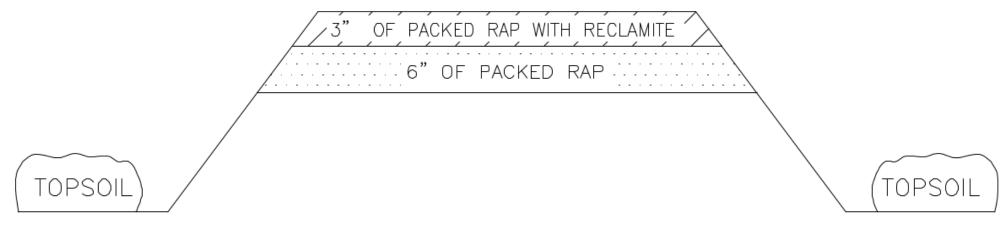
WE WIND UP WITH 2 PACKED LAYERS. ONE WITH REJUVINATOR AND ONE WITHOUT TO FORM THE BASE OF THE ROAD.
